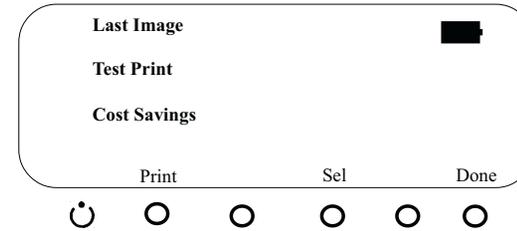
Press PRINT to obtain a printout of the most recent exam. Printing takes about one minute. See Figure 4 for an illustration of the printout.
