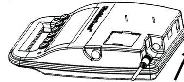
To charge a battery, plug the charger into an electrical outlet. Remove the label covering the battery contacts and slip the battery into the recess on the top of the charger. Fully charging the battery may take up to 6 hours.
