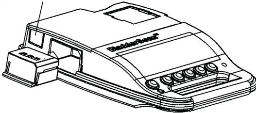
To remove the battery, push the battery release button.
