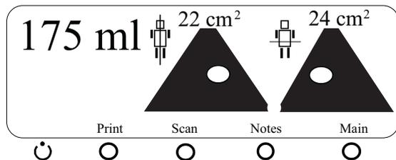
When the bladder images are completely contained in both scan planes, the measurement results are accurate. Pressing either the PRINT or MAIN button completes the scanning procedure and stores the measurement results in the instrument's memory.
